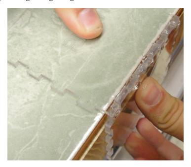
2. Place a line of glue along the edges that the front and right side share with the front. Snap the front into place and hold until glue has dried. Make sure the latch is on the inside of the box.
